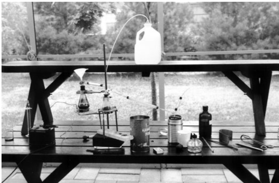
Figure 2. Setup for preparing \text{Cl}_2 and reacting it with red phosphorus, sometime in 1966-1967, in our screened backyard patio. The leftmost flask contained \text{KMnO}_4 to react with aqueous \text{HCl} added through the funnel controlled by a pinch clamp. The \text{Cl}_2 was dried by passage through \text{CaCl}_2 then directed onto \text{P}_4 in the flask on the ring stand. Because no running water was available, the water to cool the \text{PCl}_3 condenser was siphoned from the recycled milk jug and deposited into the waste can labeled "Hawaiian Punch". The receiver for \text{PCl}_3 was immersed in ice in the thermos bottle. The alcohol lamp allowed auxiliary heating for the phosphorus. Note rubber stoppers everywhere.
